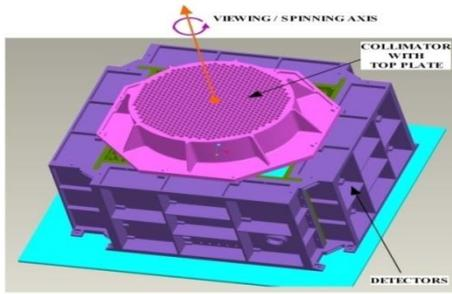
Figure 1 Instrument configuration.
