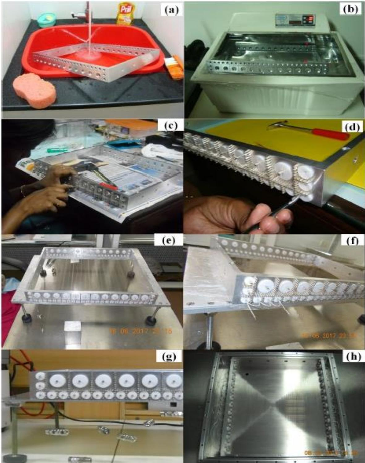
Figure : 13 Different steps involved in the wiring.(a)Soap water cleaning,(b)Ultrasonic cleaning,(c)Cathode pin fixing,(d) Teflon bushes fixing(e) Cathode wiring, (f) Antianode loop wiring(g) Anode wiring, (h) The completed frame.
