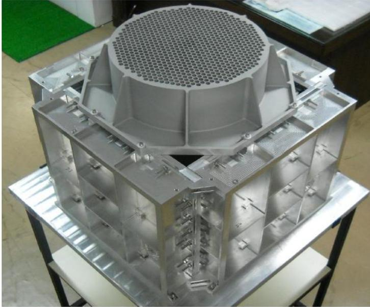
Figure : 12 POLIX four detector and collimator assembly.
