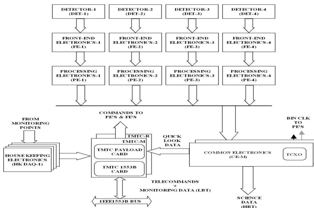
Figure : 17 The block diagram of Polarimeter electronics.
