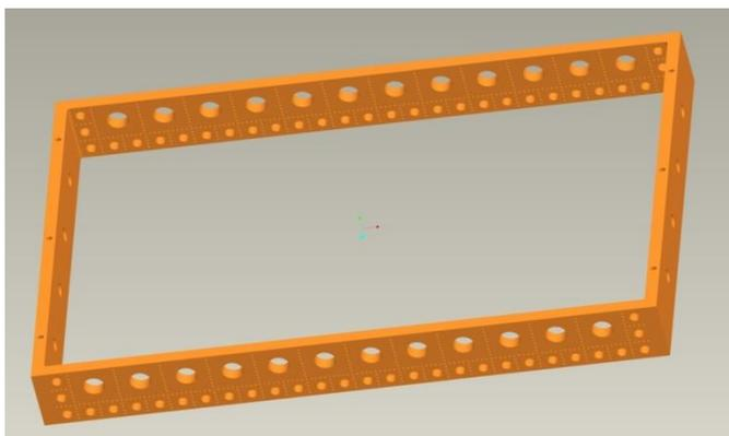
Figure : 4 The detector wire frame
