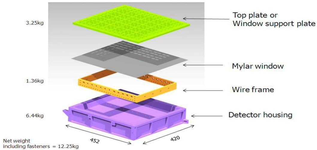
Figure: 3 Exploded view of the detector showing the different parts. The individual weights are also shown
