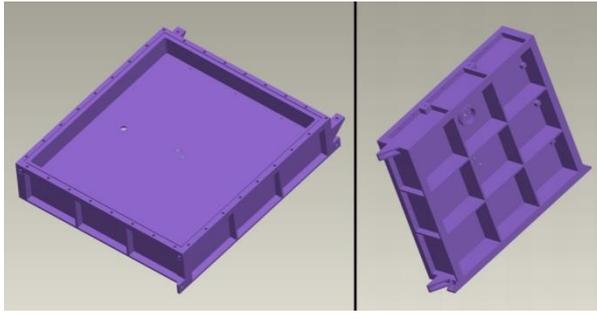
Figure : 8 Top view of the detector housing (left) and bottom view of housing (right)
