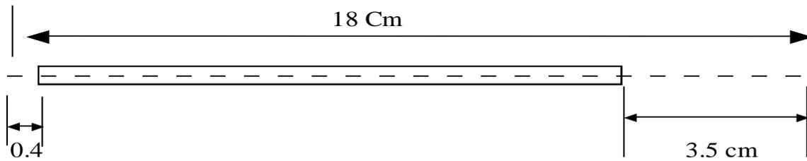
strip off 0.4 cm on anode side and 3.5cm on the feed thru side
