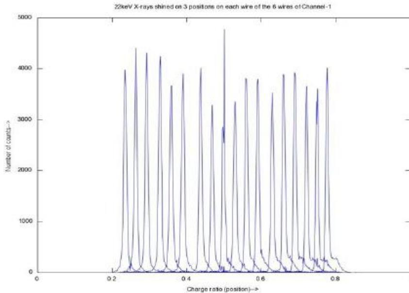
Figure : 18 Charge ratio vs position at 18 positions along the anode wire.
