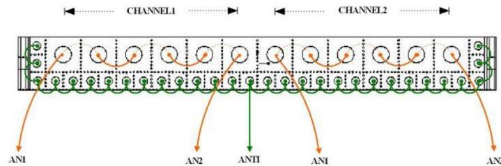
Figure :7 The detector internal wiring
