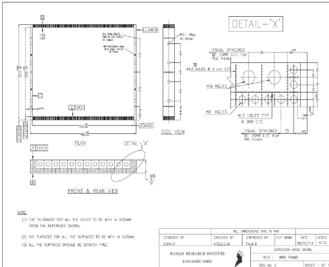
Figure: 6 Mechanical diagram of the Detector
