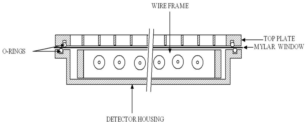
Figure : 10 O-ring positions in assembled view
