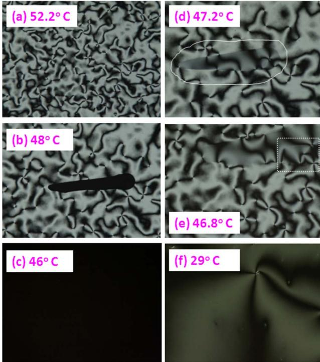
FIG. 1. (Color online) Photomicrographs of the textures around the anchoring transition temperature in CCN-47 between crossed polarizers at (a) 52.2, (b) 48, and (c) 46 °C, all under zero field. Textures in the same region under an electric field 0.29 V/ $\mu$ m, as photographed at (d) 47.2, (e) 46.8, and (f) 29 °C. White dotted lines in Fig. 1(d) enclose a domain with tilted director. Cell thickness 5.2  $\mu$ m.
