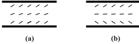
FIG. 4. Schematic diagram illustrating the director orientations near the two surfaces and the midplane of the cell below the anchoring transition of type 2 corresponding to (a) the even and (b) the odd solutions of  $\psi(z)$ .
