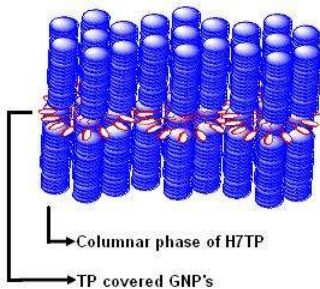
Figure 31. A schematic diagram illustrating arrangement of TP-GNPs in the inter domain spacing formed between the discotic columns.
