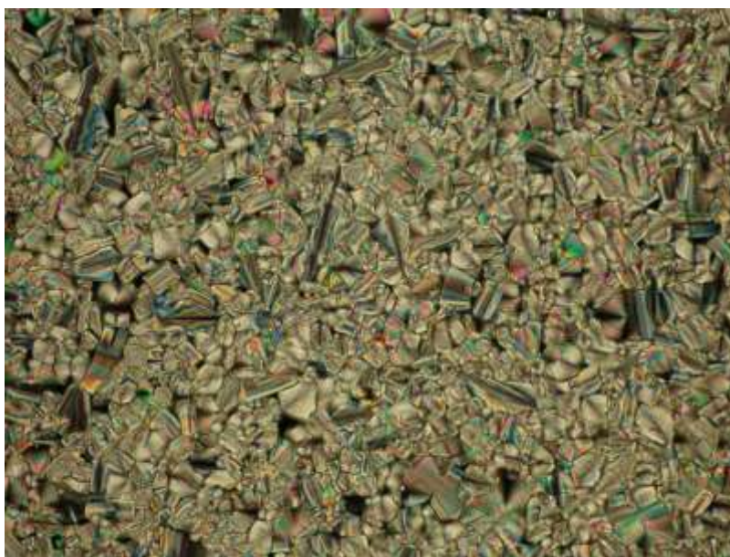
Figure 11. Optical photomicrograph of 17b obtained with a polarizing microscope on cooling from the isotropic liquid at 100 °C (crossed polarizers, magnification X 200).
