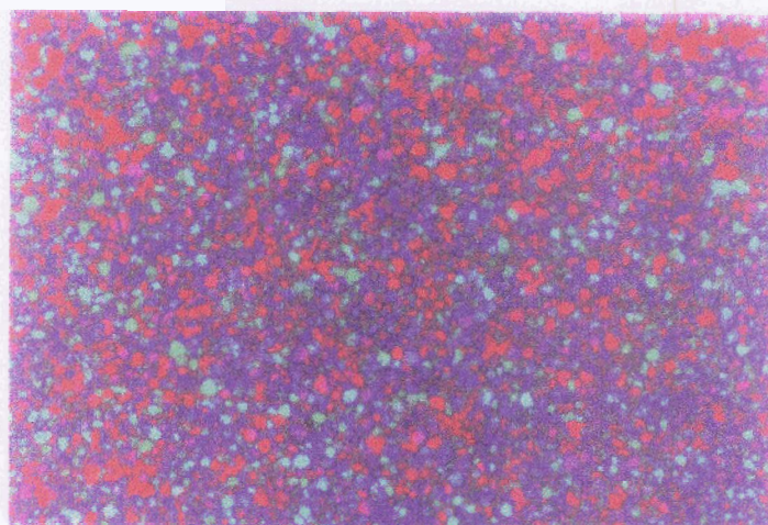
Fig. 7.4. Optical photomicrograph of the blue phase of compound 7.B.1 close to the isotropic phase.
