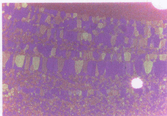
Fig. 7.2. Optical photomicrograph of the blue phase of compound 7.A.1 close to the isotropic phase.
