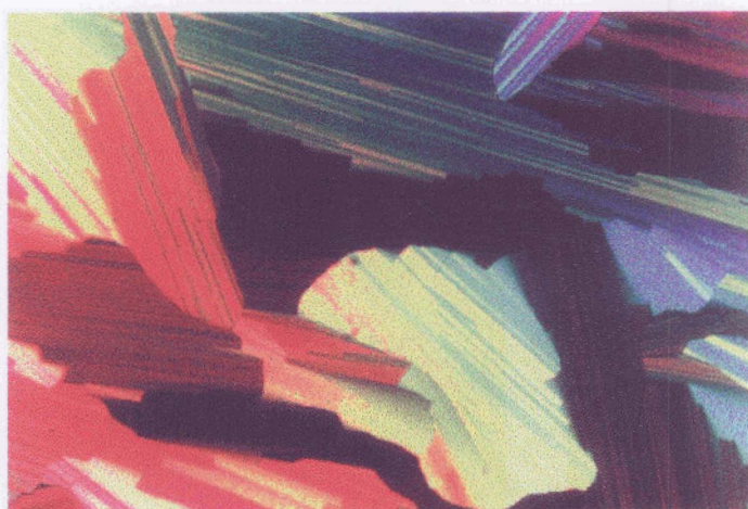
Fig. 3.7. Optical photomicrographs obtained for compound 3.B.2 (a) a B_1 mesophase growing from the nematic phase and (b) completely formed uniform mosaic texture of the B_1 phase.
