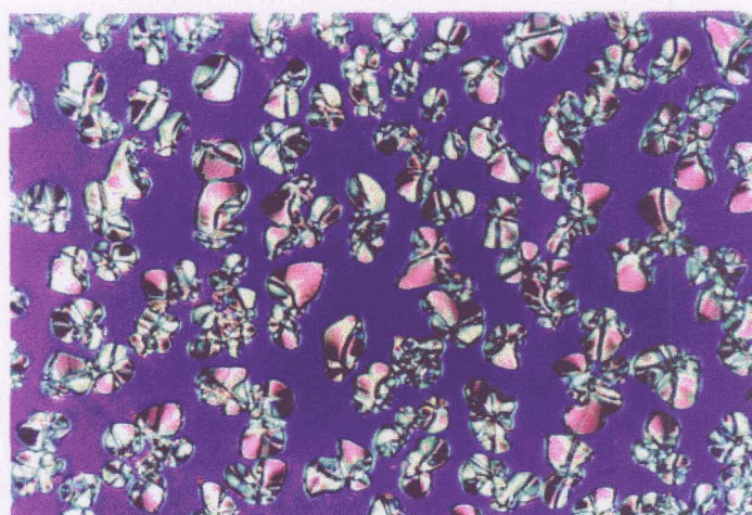
Fig. 3.10. Photomicrographs obtained for compound 3.B.10 , (a) the unusual textural pattern obtained in the nematic phase and (b) small broken fan-like texture of B_2 phase developing from a homogeneously aligned nematic phase.
