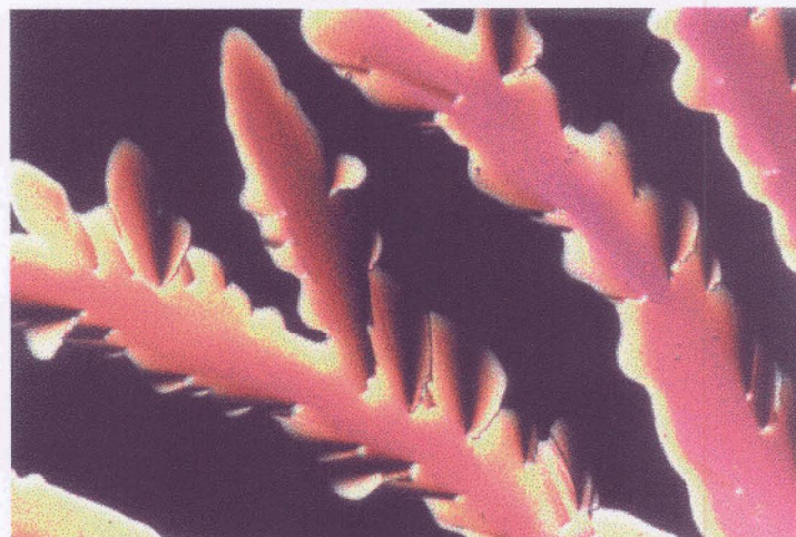
Fig. 3.18. An unusual texture of the B_{X5} mesophase obtained on cooling the isotropic liquid of compound 3.F.5.
