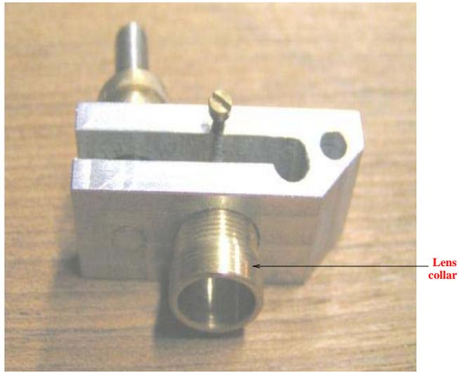
Figure 2.15: Laser-lens module front view
