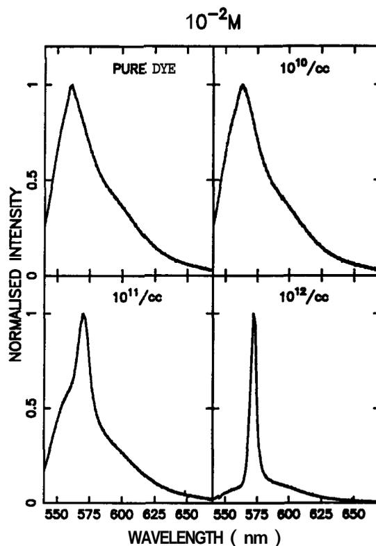
Figure 9.10: Emissions from the same dye at a concentration of  $10^{-2}M$  under three-dimensional pumping conditions, at various scatterer concentrations at a pump energy of  $600 \mu J$ . The emission is always monomodal.
