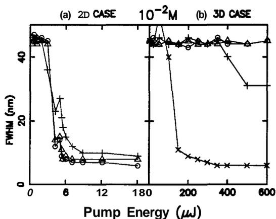
Figure 9.11: FWHM of the emission spectrum as a function of pump energy of (a) the 2D pumped system and (b) the 3D pumped system.  $o$  : Pure dye,  $\Delta$  :  $10^{10}/cc$ ,  $+$  :  $10^{11}/cc$ ,  $x$  :  $10^{12}/cc$ . Note that the X-axis is scaled differently in the two cases.
