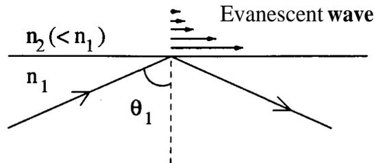
Figure 9.1: *The formation of an evanescent wave at an interface between two dielectrics. The ray is incident onto the interface at an angle greater than the critical angle from the medium with the higher refractive index. Evanescent wave forms inside the rarer medium, propagates along the interface, and has an amplitude that decays exponentially within a wavelength in the direction normal to the interface.*
