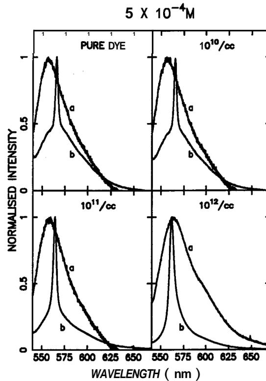
Figure 9.3: Emission spectra of the dye at a concentration of  $5 \times 10^{-4} M$ , at various scatterer concentrations, under evanescent pumping. Curve (a) is the spectrum at pump energy  $2 \mu J$  and (b) at  $9 \mu J$ . A marked change in the spectrum at  $9 \mu J$  is seen in the case of the scatterer concentrations  $10^{11}/cc$  and  $10^{12}/cc$ .
