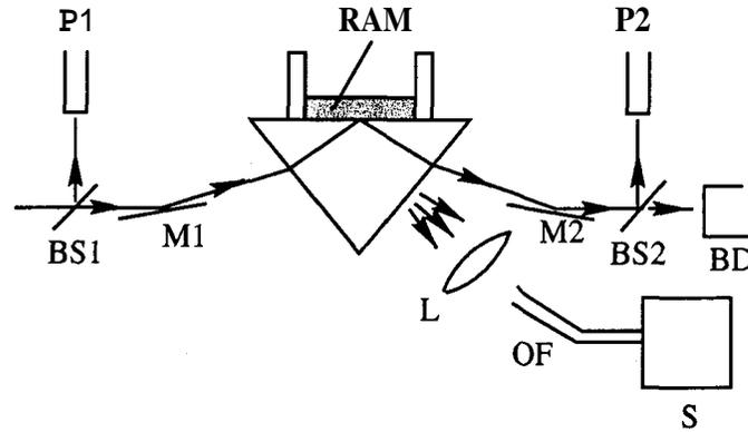
Figure 9.2: *Experimental setup for studying the emission spectrum from a random amplifying medium pumped by an evanescent field. BS1, BS2 : Beamsplitters, M1, M2 : Mirrors, P1, P2 : Probes of an energy ratiometer, L : Lens, OF : Optic Fibre, BD : Beam Dump, S : Spectrometer, RAM : Random Amplifying Medium.*
