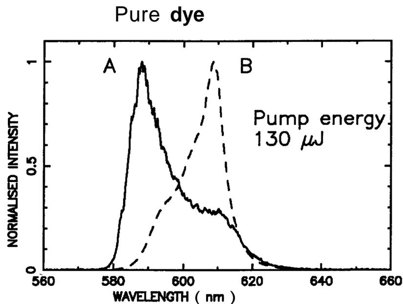
Figure 8.2: Experimentally observed emission spectra at the two ends of the diode, with homogeneous amplifying medium. End A is the low concentration end.
