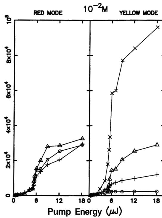
Figure 9.9: Peak intensity of emission in the two modes as a function of pump energy at various scatterer concentrations.  $o$  : Pure dye,  $+$  :  $10^{10}/cc$ ,  $\Delta$  :  $10^{11}/cc$ ,  $x$  :  $10^{12}/cc$ .
