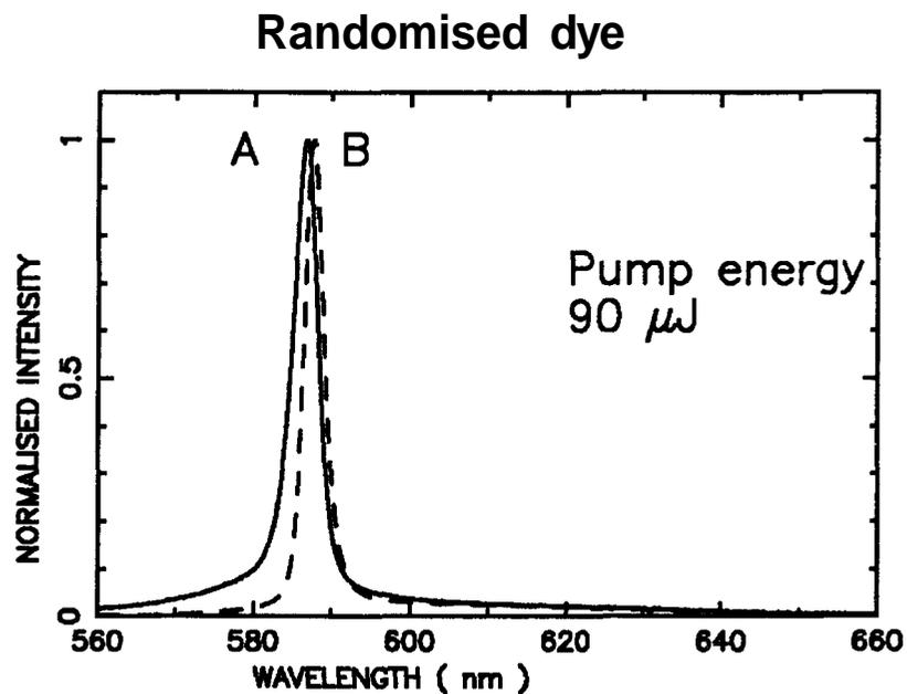
Figure 8.3: Experimentally observed emission spectra from the diode, with scatterers in the amplifying medium.
