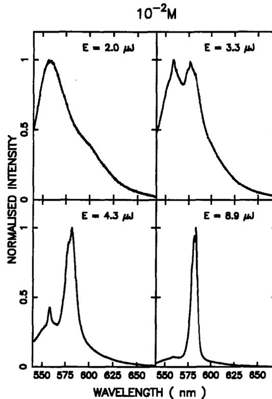
Figure 9.6: *Bichromatic emission seen from the pure dye of concentration  $10^{-2}M$  at various pump energies, under evanescent pumping. The system lases in the red mode (583nm) at high pump energies.*
