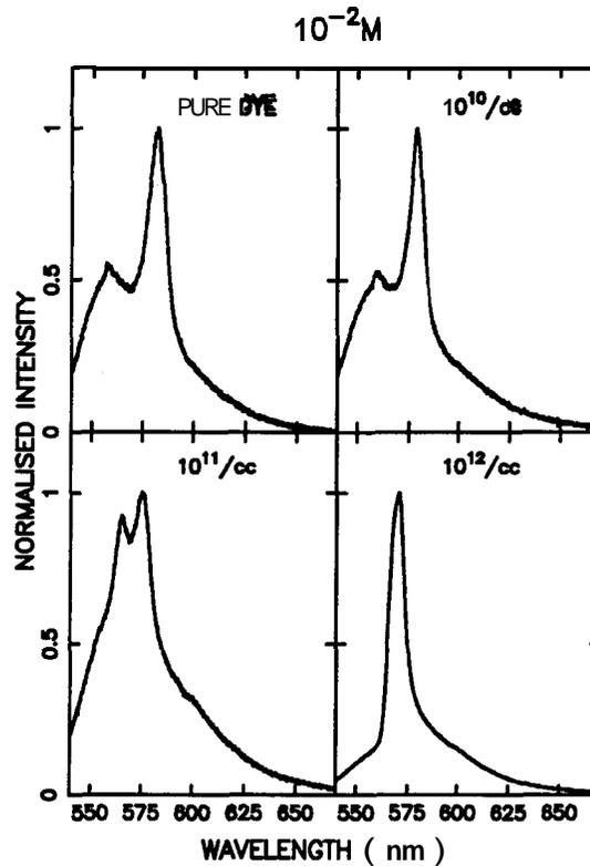
Figure 9.7: Normalised emission spectra from a dye of concentration  $10^{-2}M$  with various scatterer concentrations at a pump energy of  $4\mu J$ , under evanescent pumping. Clearly, the addition of scatterers forces the system to lase in the yellow mode ( $570nm$ ), in contrast to the emission from the pure dye shown in figure 9.6. The competition between the two modes upon addition of disorder is obvious from the four subplots.
