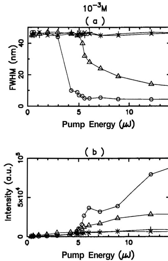
**Figure 9.5:** Variation of (a) FWHM and (b) Peak Intensity of emission with pump energy at a dye concentration of  $10^{-3}M$ .  $x$  : Pure dye,  $+$  :  $10^{10}/cc$ ,  $\Delta$  :  $10^{11}/cc$ ,  $\circ$  :  $10^{12}/cc$ .
