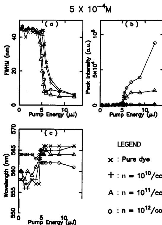
Figure 9.4: Details of the emission profiles of the dye at a concentration of  $5 \times 10^{-4} \text{M}$ , under evanescent pumping. The subplots show, as a function of the pump energy, (a) the reduction of FWHM, (b) the peak intensity, and (c) the wavelength of peak emission. The legend is explained in the figure. The reduction in FWHM and the enhancement in emission intensity upon addition of scatterers is obvious from the figure.
