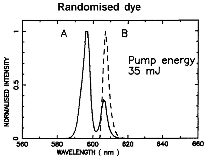
Figure 8.5: *Simulated spectra for a 1-d exponentially graded gain medium with random scatterers.*
