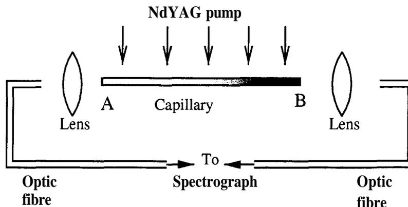
Figure 8.1: Schematic of the experimental setup. The capillary is pumped longitudinally and the emissions from the two ends are analysed.
