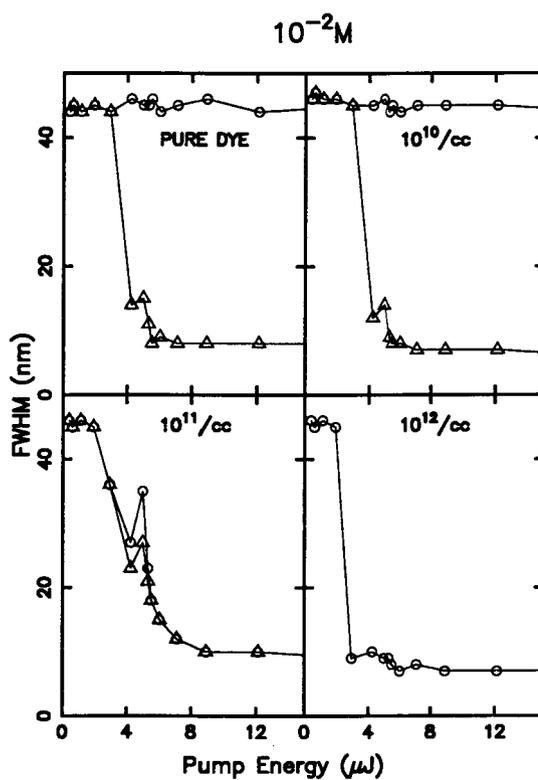
**Figure 9.8:** Variation of FWHM, as a function of pump energy, of the two modes ( $\circ$  = yellow mode,  $\triangle$  = red mode) of the bichromatic emission seen from the dye of concentration  $10^{-2}M$ . The effect of addition of scatterers is evident from the four subplots. The broadband yellow mode starts narrowing as scatterers are added. The red mode is absent in the case of scatterer concentration of  $10^{12}/cc$ , and the system lases in the yellow mode.
