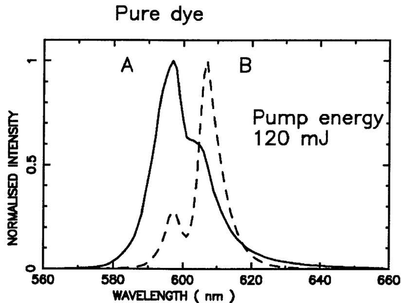
Figure 8.4: Simulated spectra for a 1-d exponentially graded gain medium. End A is the low concentration end.
