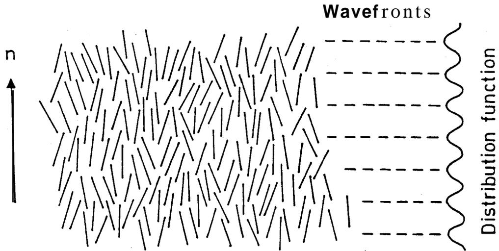
Figure 3: Schematic representation of the molecular arrangement in smectic A phase (after Leadbetter<sup>3</sup>).
