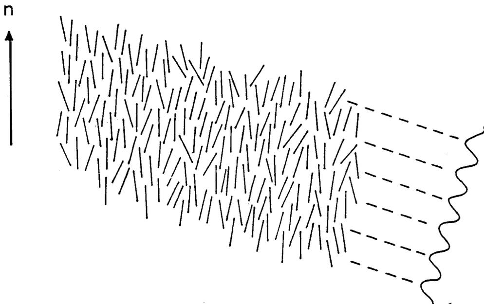
Figure 4: Schematic representation of the molecular arrangement in smectic C phase (after Leadbetter<sup>3</sup>).
