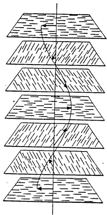
**Figure 2:** Schematic representation of the molecular arrangement in chiral nematic phase. (after Chandrasekhar<sup>4</sup>).
