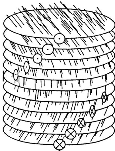
**Figure 5:** Schematic representation of the molecular arrangement in chiral smectic C phase with the direction of spontaneous polarisation (after Escher<sup>76</sup>).
