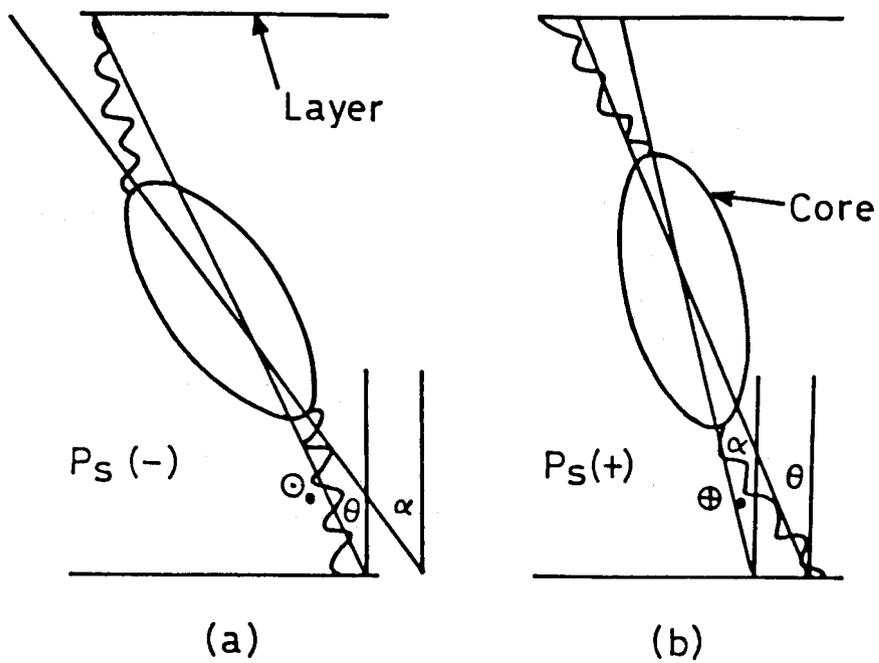
Figure 8: Two possible **tilt** orientations of a molecule in chiral smectic C phase (after Goodby et al.<sup>73</sup>).
