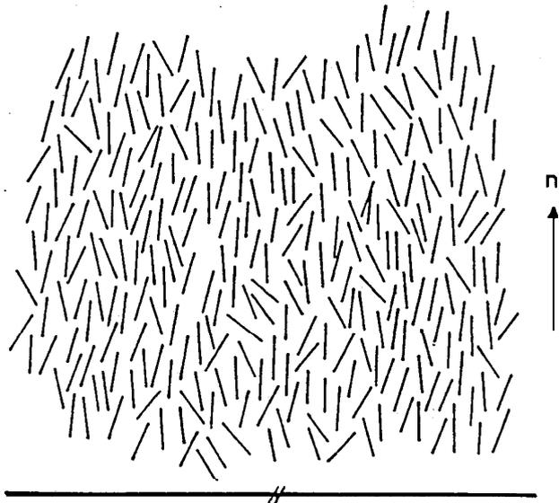
**Figure 1:** Schematic representation of the molecular arrangement in nematic phase (after Leadbetter<sup>3</sup>).
