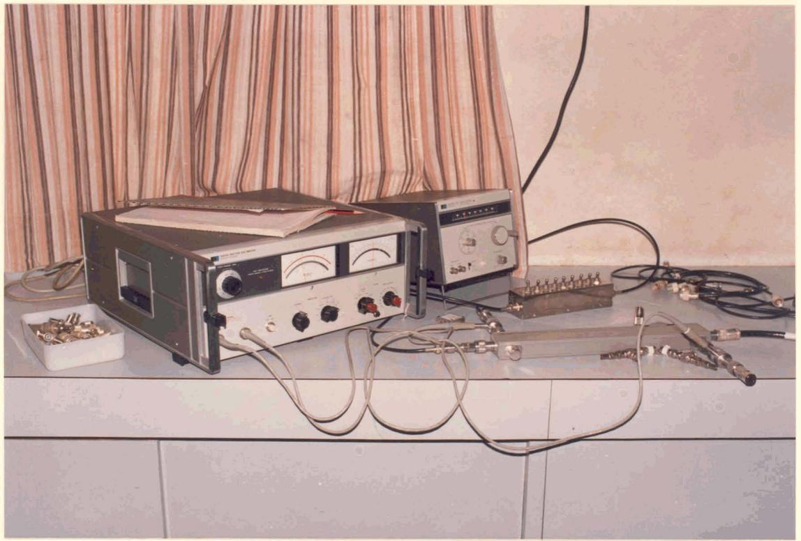
**Figure 4.10 Co-axial Cable Phase Equalisation
