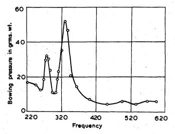
Figure 4. Relation between bowing pressure and pitch (with mute).
